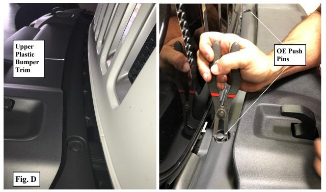
**<u>Step 6:</u>** Carefully remove the **OE** front bumper from the vehicle.
